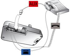
Figure 16: Connecting to a GN1000 Remote Handset Lifter
